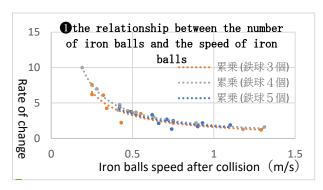
**1** The relationship between the number of iron balls and the speed of iron balls. According to this graph, we found the condition with the most speed was the device with 4 iron balls.
